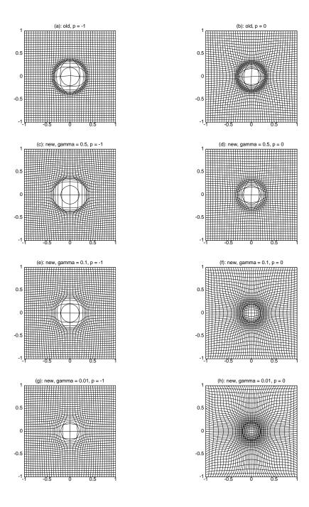
Fig. 7. Adaptive meshes are obtained for Example 5.1 with the harmonic mapping (p=-1) and arclength (p=0) monitor functions. Desirable mesh point concentration is around the circle  $x^2+y^2=0.2^2$  (the bold solid circle).
