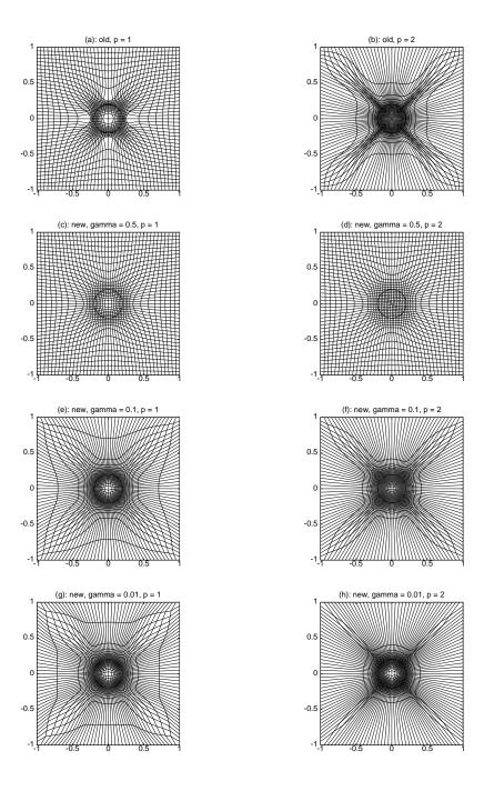
FIG. 8. Adaptive meshes are obtained for Example 5.1 with the Winslow-type (p=1) and strong concentration (p=2) monitor functions. Desirable mesh point concentration is around the circle  $x^2+y^2=0.2^2$  (the bold solid circle).
