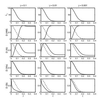
FIG. 5. Normalized mesh densities (solid lines) obtained with the new functional for a monitor function (dashed lines) such that  $\lambda_1(r) = 1 + \exp(-(r - r_{\lambda})^2/a)/a$  (a = 0.01,  $r_{\lambda} = 0$ ) for different choices of  $\lambda_2$  and  $\gamma$  (q = 2).
