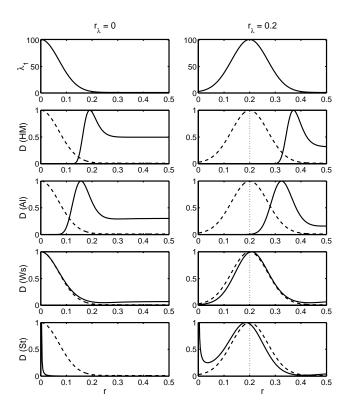
FIG. 3. Normalized mesh densities obtained with the traditional functional for different monitor functions defined in (2.2) and with  $\lambda_1(r) = 1 + \exp(-(r - r_{\lambda})^2/a)/a$  (a = 0.01) that has its maximum located at  $r_{\lambda} = 0$  (left column) and  $r_{\lambda} = 0.2$  (right column). The top plot depicts  $\lambda_1(r)$ . For guidance, we plot, along with the normalized densities (solid lines), the normalized curve for  $\lambda_1(r)$  (dashed lines).
